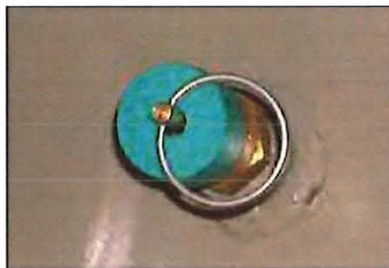
Figure 4. Automatic Pressure relief valve.
