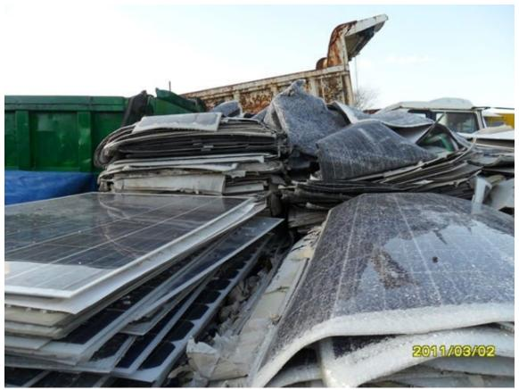
Figure 4: The mangled PV panels in this picture illustrate the nature of broken solar panels; the glass cracks but the panel is still in one piece. Image Source: <a href="http://img.alibaba.com/photo/115259576/broken">http://img.alibaba.com/photo/115259576/broken</a> solar panel.jpg
