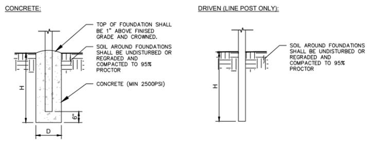
① FENCE POST DIMENSIONS ARE LISTED BELOW AND ALL POSTS SHALL BE IN ACCORDANCE WITH ASTM F1083, SCHEDULE 40 OR ASTM F1043, GROUP C.
