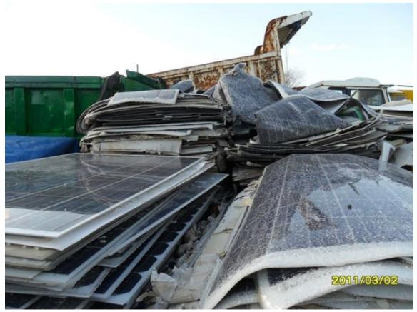
Figure 4: The mangled PV panels in this picture illustrate the nature of broken solar panels; the glass cracks but the panel is still in one piece. Image Source: <u>http://img.alibaba.com/pho-to/115259576/broken\_solar\_panel.jpg</u>
