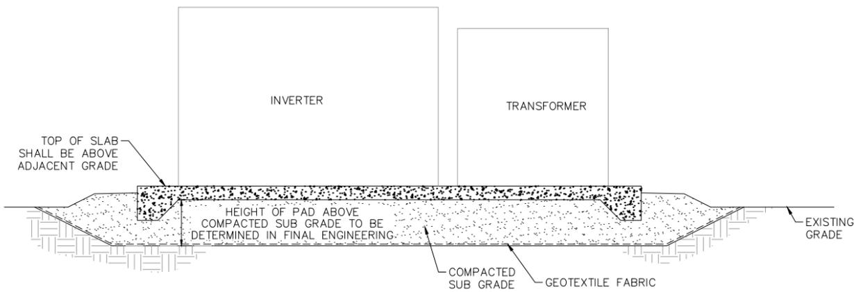
10 EXAMPLE EQUIPMENT PAD ELEVATION DETAIL
