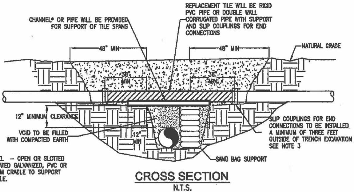
\*CHANNEL - OPEN OR SLOTTED CORRUGATED GALVANIZED, PVC OR ALUMINUM CRADLE TO SUPPORT DRAIN TILE.
