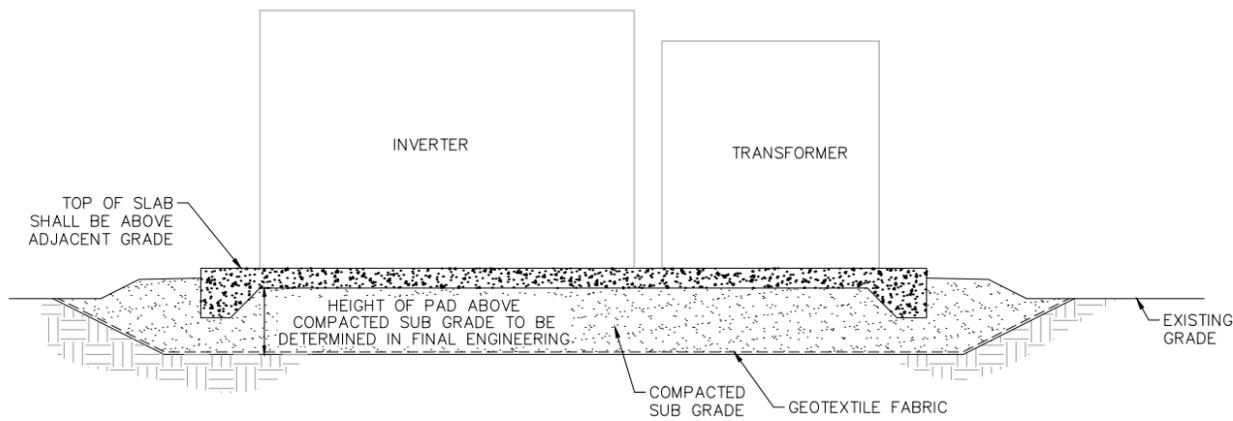
10 EXAMPLE EQUIPMENT PAD ELEVATION DETAIL
