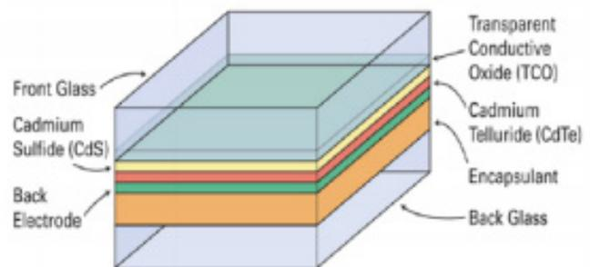
*Figure 3: Layers of a common frameless thin-film panel (CdTe). Many thin film panels are frameless, including the most common thin-film panels, First Solar's CdTe. Frameless panels have protective glass on both the front and back of the panel. Layer thicknesses not to scale. Image Source: [www.homepower.com](http://www.homepower.com)*
